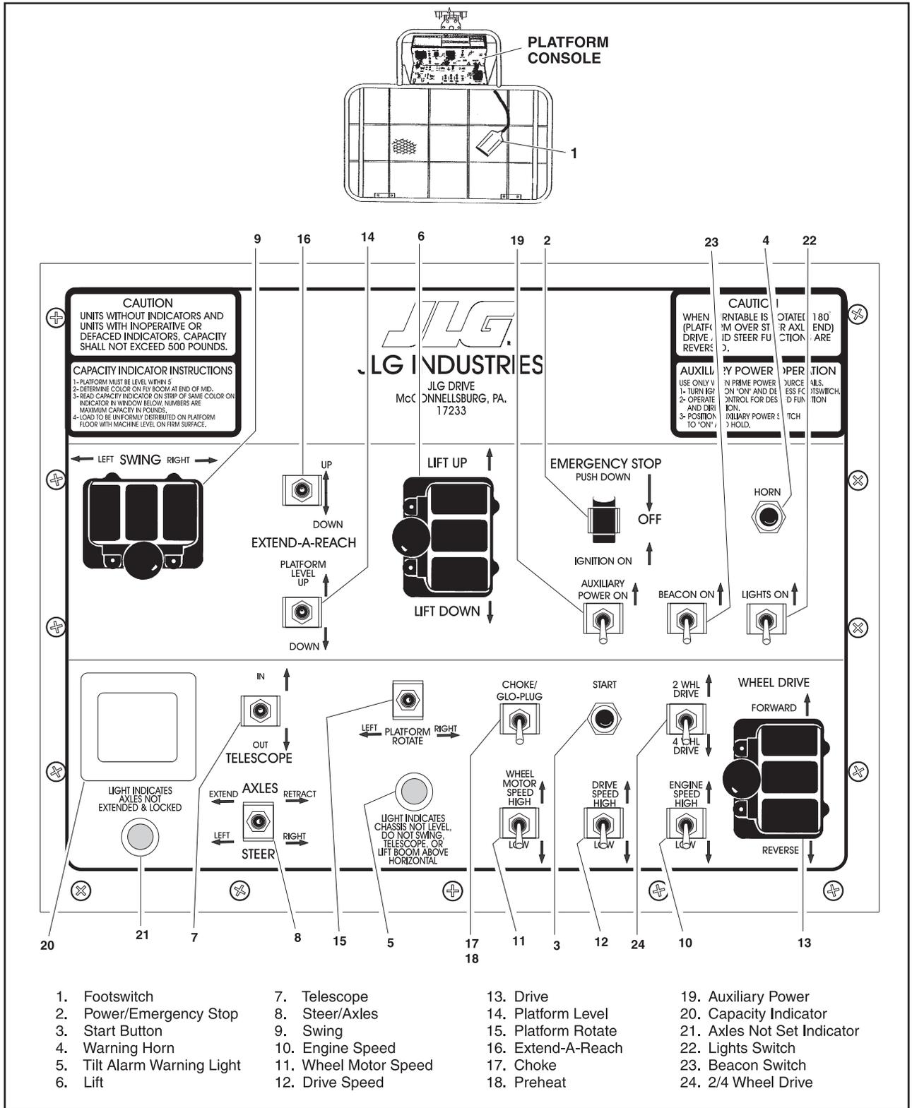
**Figure 3-10. Control Console - Prior to Sept. 91**
