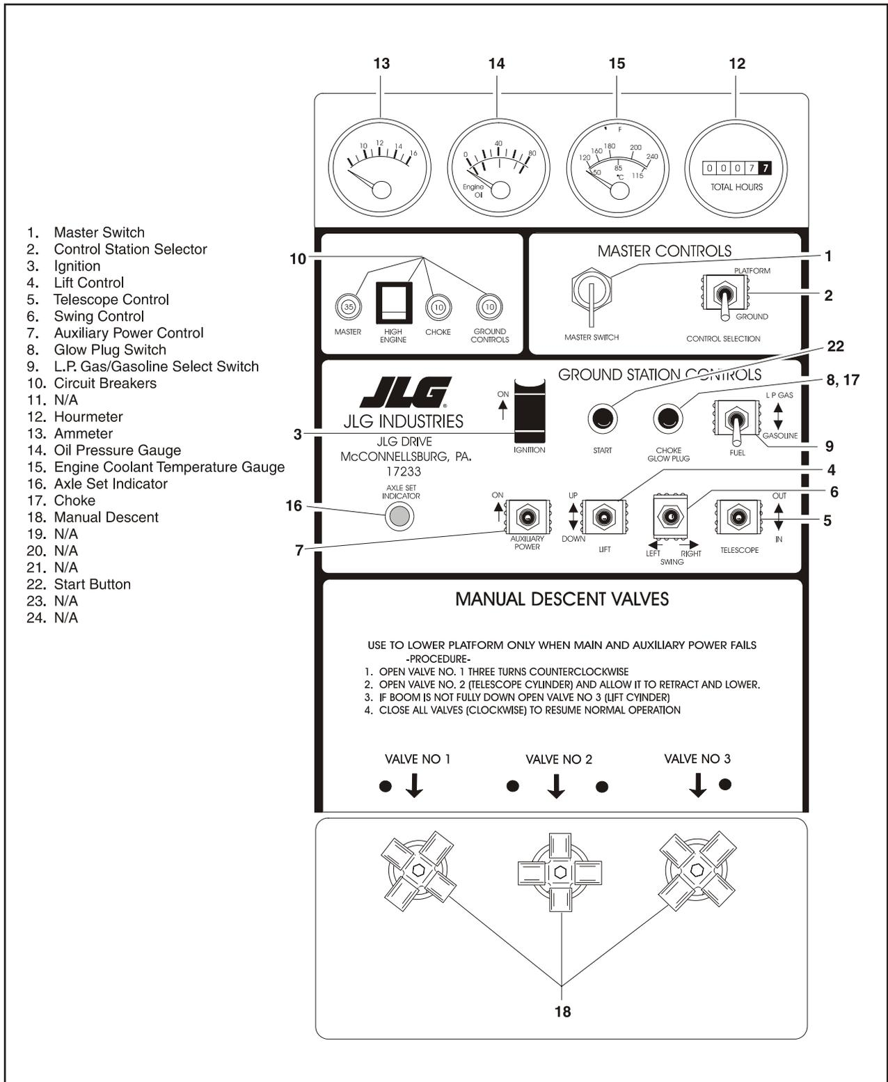
**Figure 3-6. Ground Control Station - 750 LB Capacity Machines Prior to May 1994**
