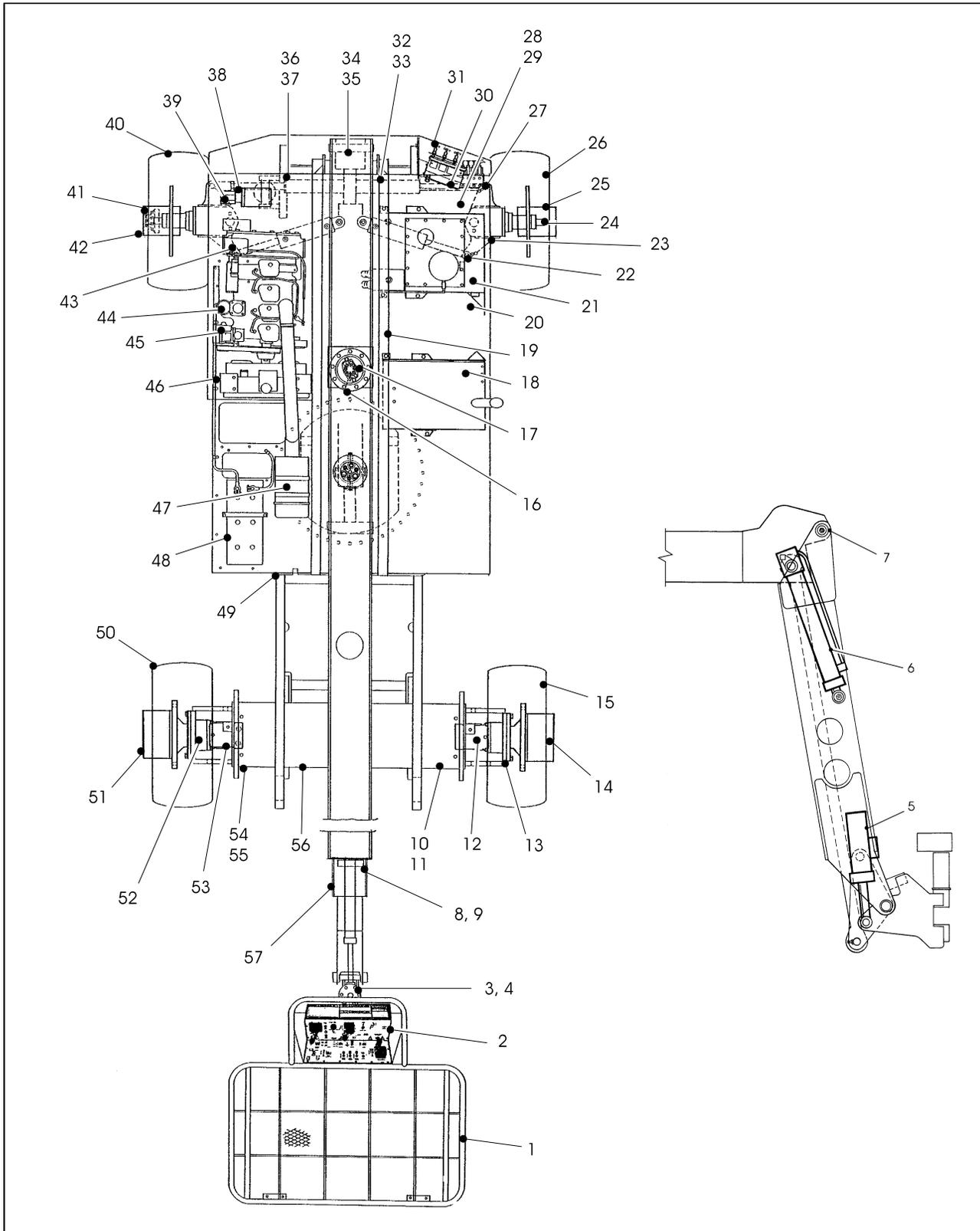
Figure 2-2. Daily Walk-Around Inspection - Sheet 1 of 4
