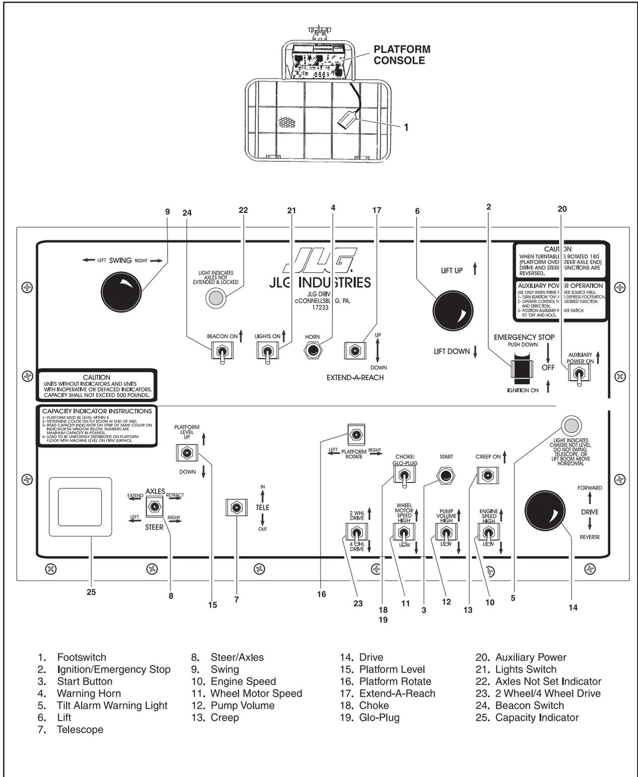
**Figure 3-14. Control Console - OEM Controllers**
