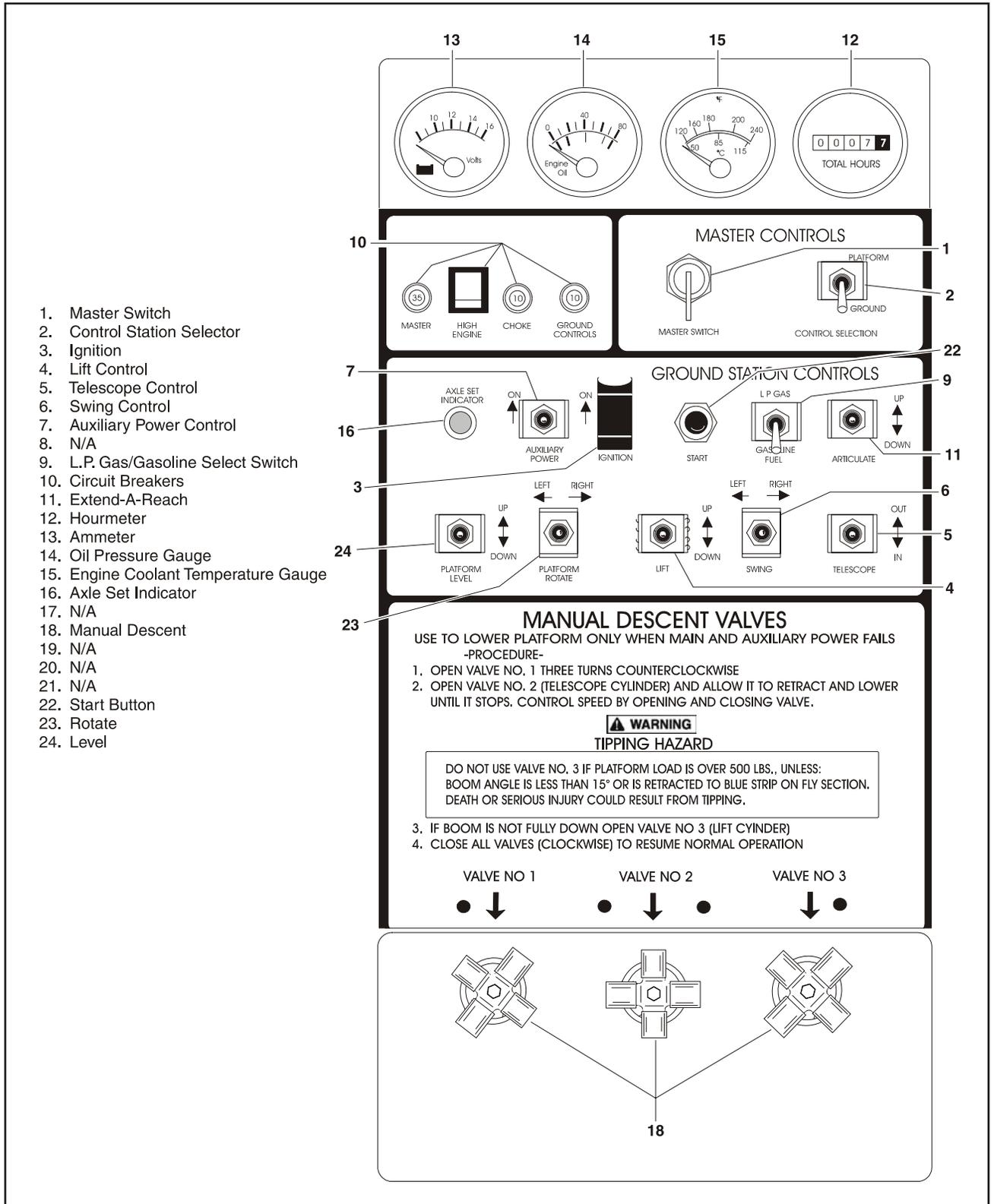
**Figure 3-4. Ground Control Station - May 1994 to Present without Hydraulic Controls**
