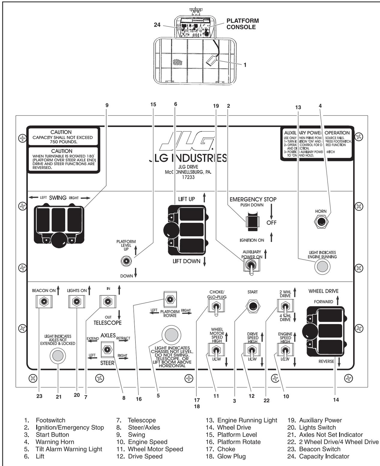
Figure 3-12. Control Console - Prior to Sept. 91 CSA Machines
