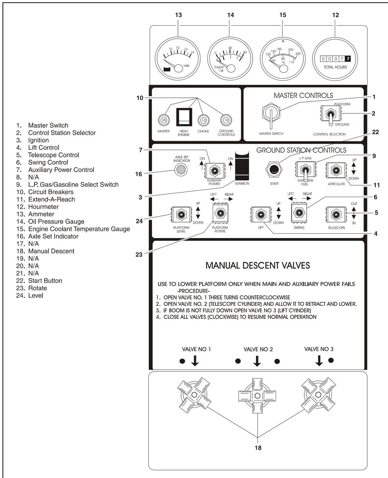
Figure 3-5. Ground Control Station - 750 LB Capacity Machines May 1994 to Present
