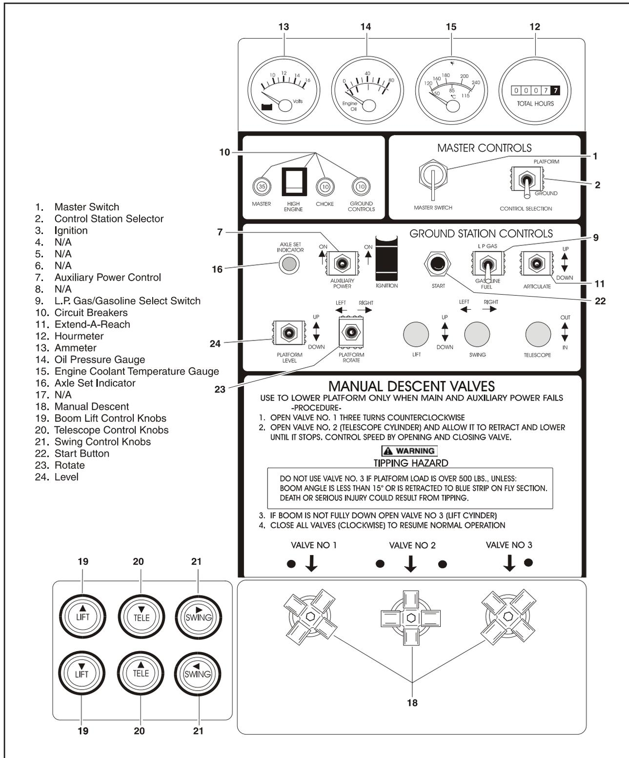
Figure 3-3. Ground Control Station - May 1994 to Present with Hydraulic Controls
