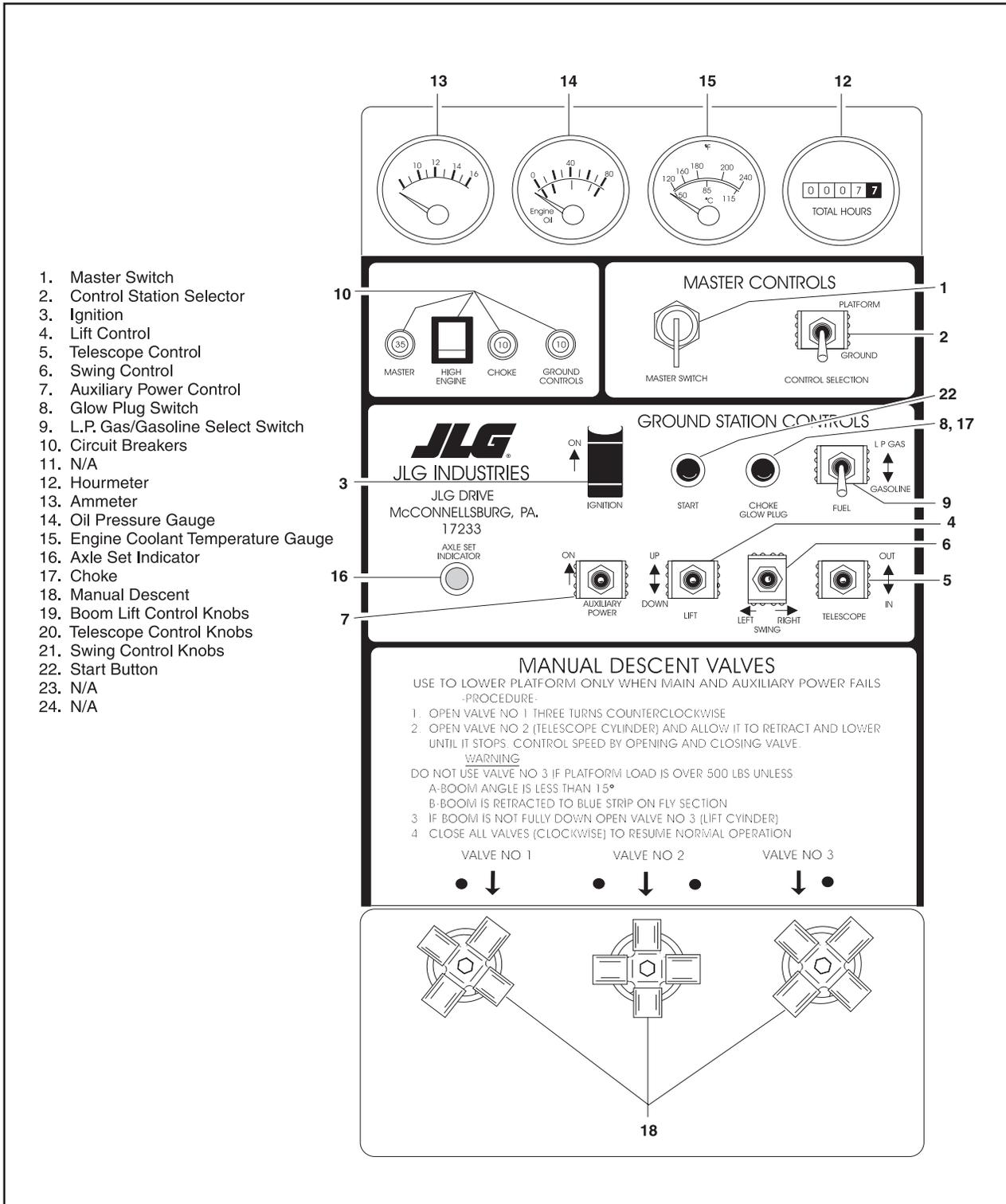
Figure 3-7. Ground Control Station - Prior to May 1994
