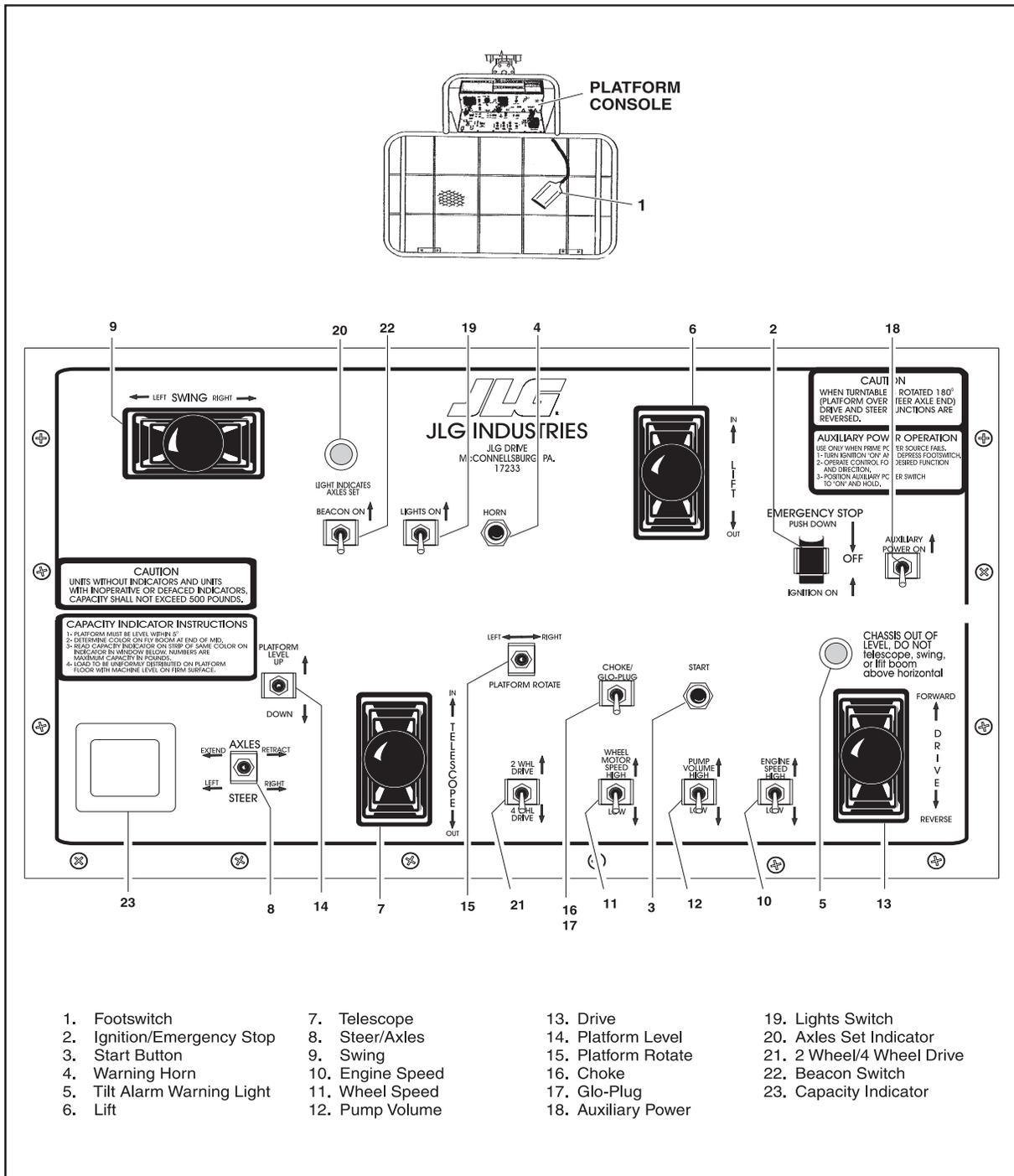
Figure 3-16. Control Console - Hydraulic Controls Prior to May 1994
