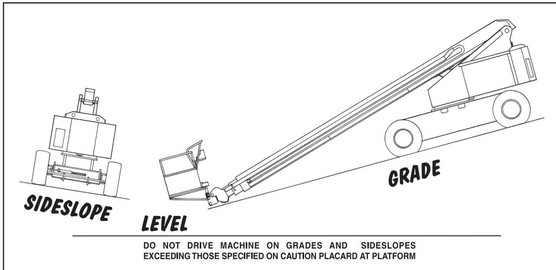
**Figure 4-1. Grade and Side Slope**
