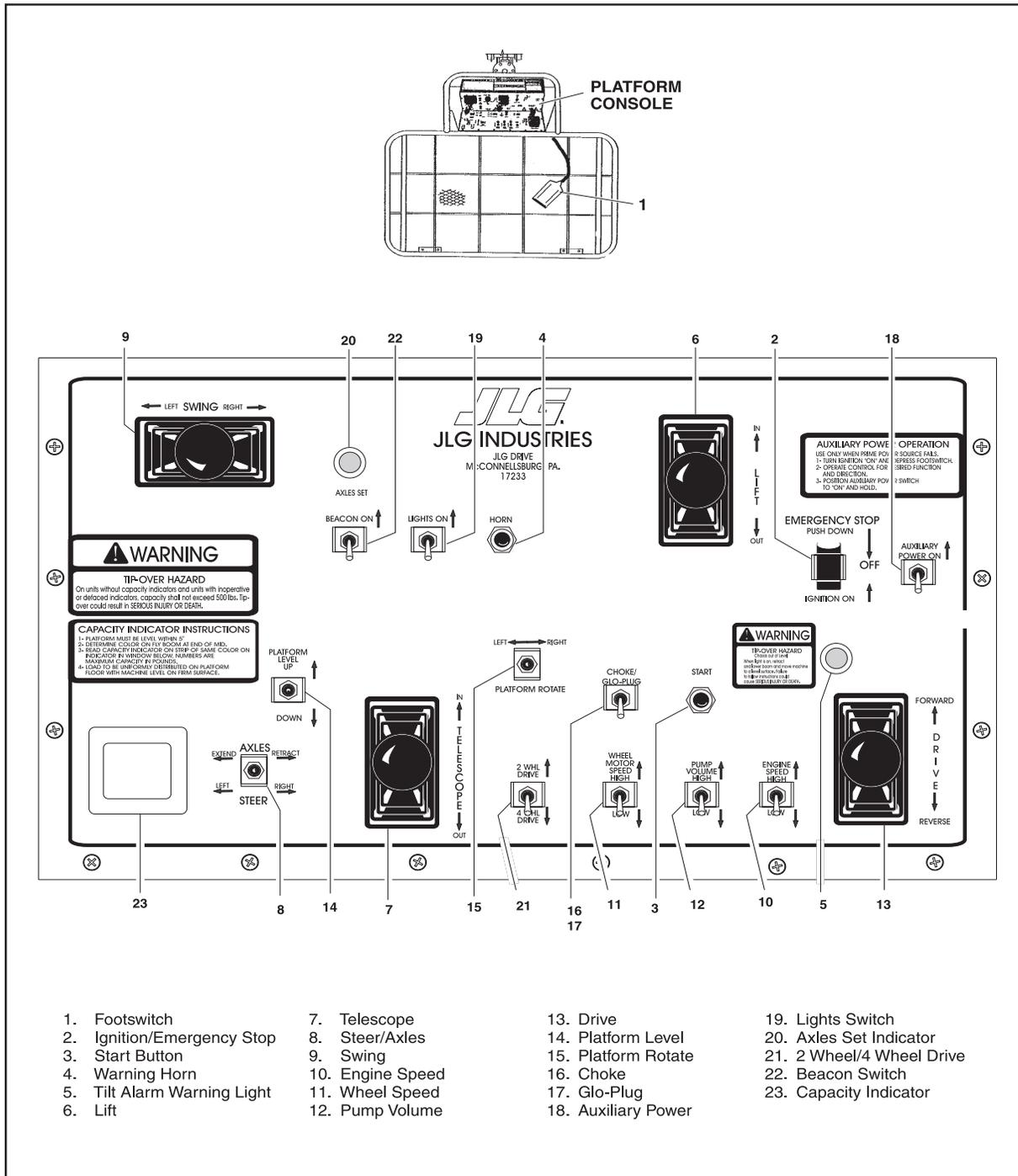
**Figure 3-15. Control Console - Hydraulic Controls May 1994 to Present**
