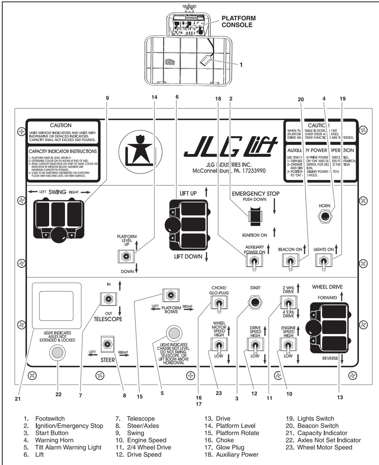
Figure 3-11. Control Console - Prior to Sept. 91 with Racine Valves
