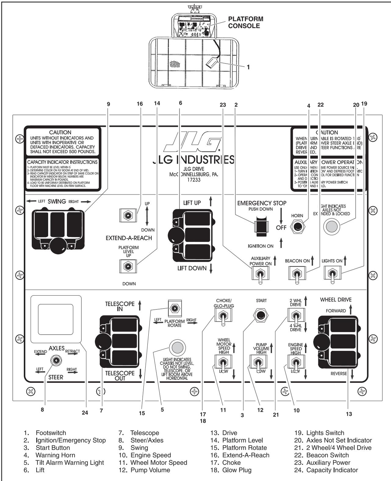
**Figure 3-13. Control Console - Prior to Sept. 91 (PQ Controllers with Proportional Telescope)**
