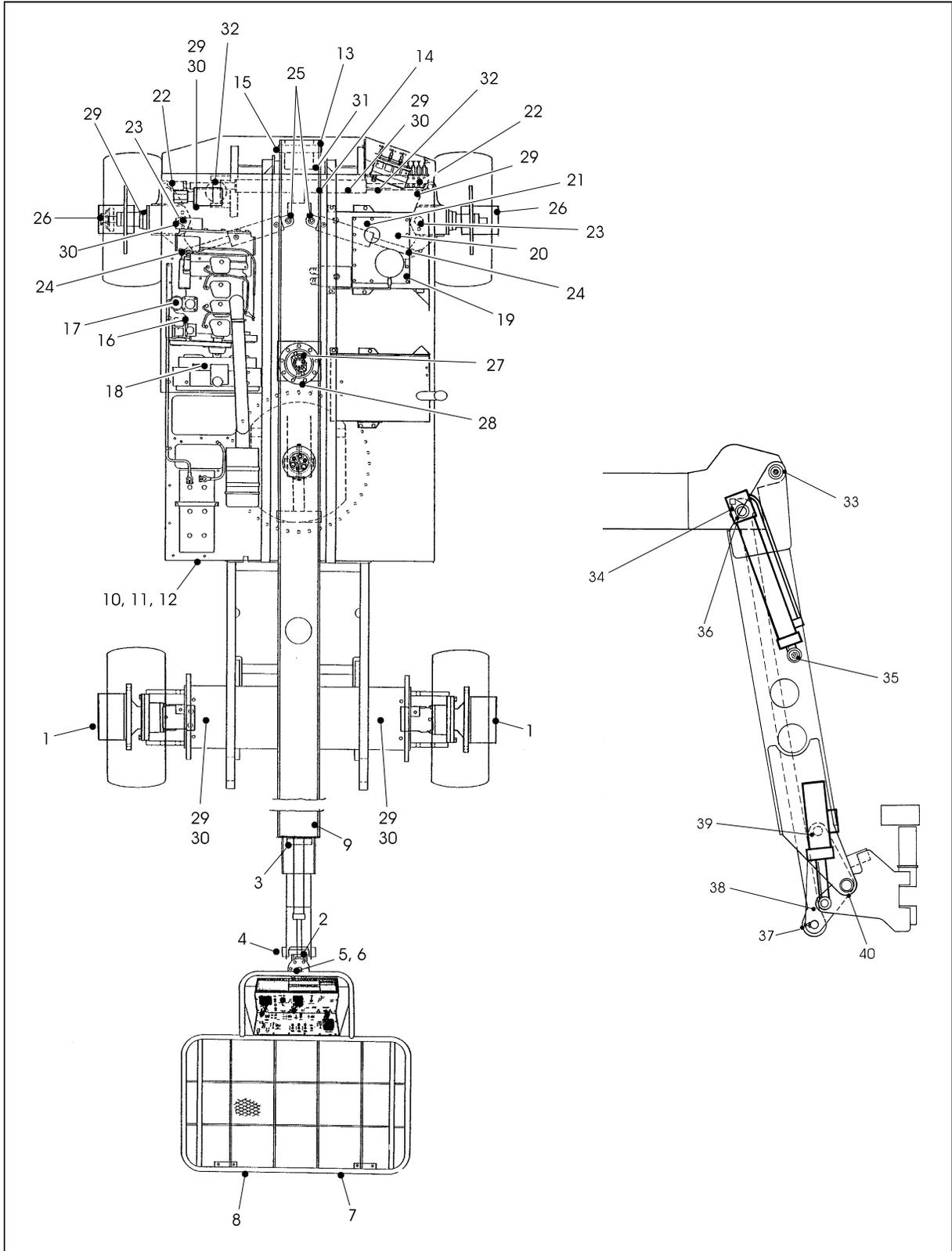
Figure 2-6. Lubrication Diagram
